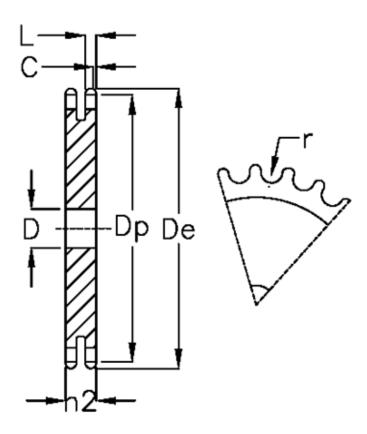
C = 4 D = 25 De = 288.6 Dp = 273.48 For chain size = 1 1/4 x 3/4 For chain type = 20 B-2 h2 = 54.6
